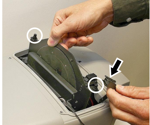
Installing a gobo wheel module
