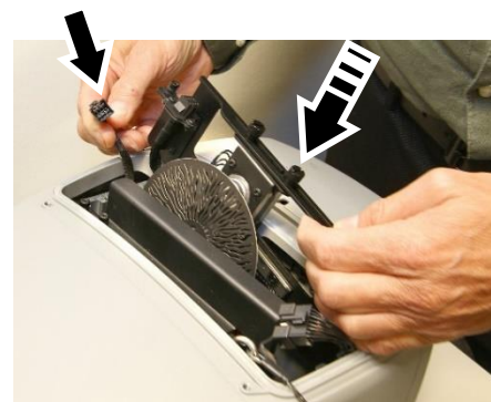
Installing an animation wheel module
