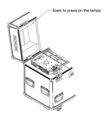
The SiP insert must be inserted into a Flightcase for 2x MAC Aura Raven XIP: P/N MAR-91515064
