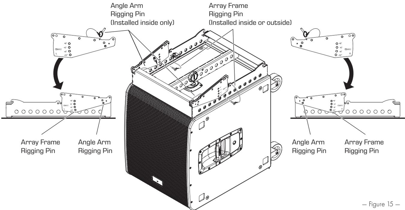
NOTE: The Stack Adapter allows loudspeakers to be installed at +6°, 0°, -6°, and -12°.
