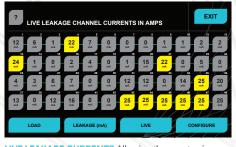
LIVE LEAKAGE CURRENTS Allowing the user to view Live RMS Earth Leakage currents across all channels. Earth Leakage levels alarms can be set by the user.
