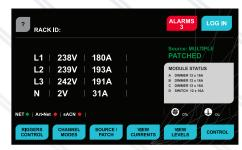
**HOME MENU** Showing real-time display of the RMS voltage and currents across all phases and Neutral, System Alarms, Rack temp, Module Status and Patch information.
