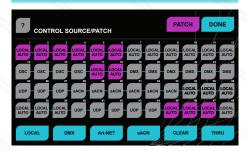
**CONTROL SOURCE/PATCH** Each individual channel can be set up to have a different control source, allowing multiple operators access to specific channels and outputs.
