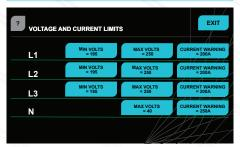
VOLTAGE AND CURRENT LIMITS Warning Limits can be set for both Voltage and Current across the incoming phases and Neutral.
