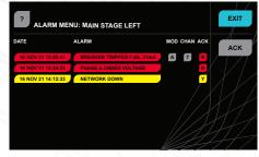
ALARMS Real time and date stamped alarms that can be viewed locally or remotely via HOUSTON X software, including loss of Control Signal, Tripped RCBOs, Over-temperature and any other system critical issues.
