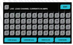
LIVE LOAD CHANNEL CURRENTS The current use is displayed for each individual channel in real-time. Alarms can be set to alert the user if they are close to exceeding their limits.
