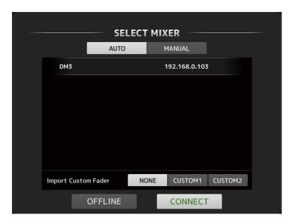
The Unit Name and IP Address of DM3 Series console found in the network are displayed in the list.
