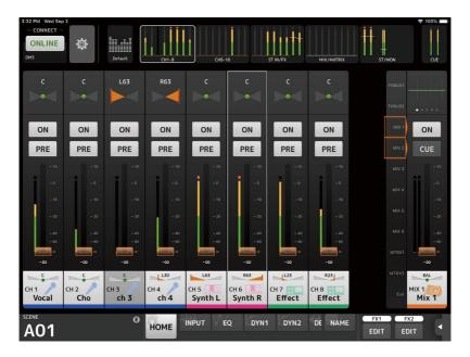
In SENDS ON FADER mode, the details area changes to display SENDS ON FADER information. Note, however, that the display does not change for channels that have no send destination.
