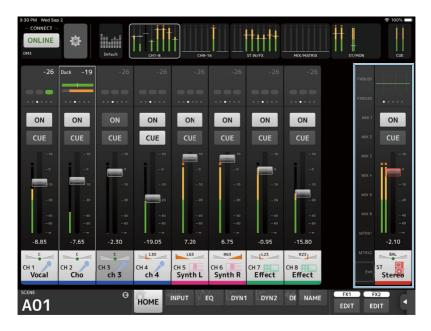
You can switch to the SENDS ON FADER mode by tapping the channel number on the left side of a strip. The selected channel is then highlighted in the channel's color. Tapping EXIT at the very bottom, or the selected channel number, restores the regular mode.
