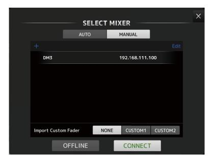
The Unit Names and IP Addresses of registered DM3 Series console are displayed in the list.
