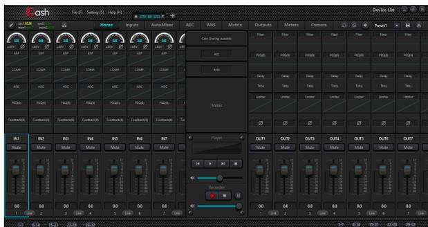
The **Dash** DSP Controller is a Windows-based, full-featured application that configures and controls the DSP hardware. Systems can be designed to perfectly match specifications and conform as requirements change or evolve. All classes of audio processing modules for signal routing and shaping are provided.
