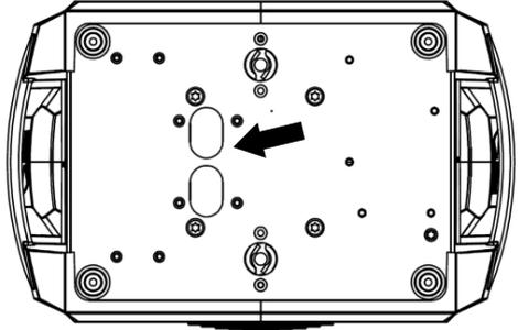
6. Remove as much slack as possible from the safety cable and fasten it to a secure anchoring point.
