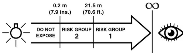
The luminaire should be positioned so that prolonged staring into the luminaire at a distance closer than 21.5 m is not expected.
