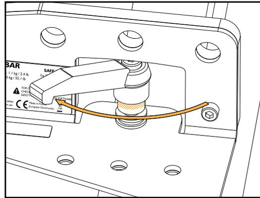
3. Release the lever and rotate it counter-clockwise.
