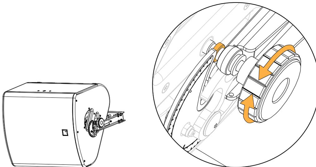
4. Push until the knobs are locked inside the spring-lock safety mechanism.
