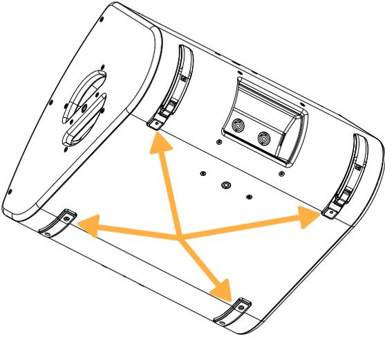
X12 features raisers that allow to change the monitor angle from 35° to 55° relative to the vertical.
