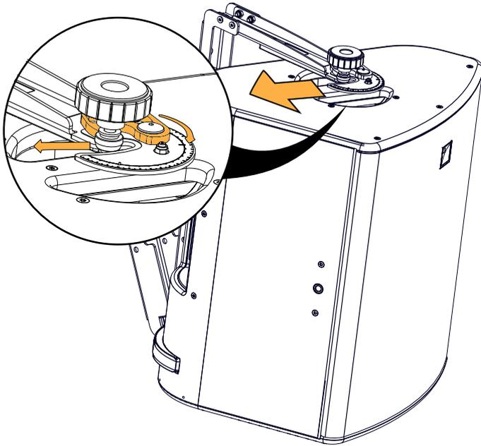
3. Remove the U-bracket and X-UTILT from the wall.
