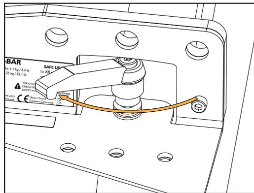
Repeat until the X-BAR is tightly secured.
