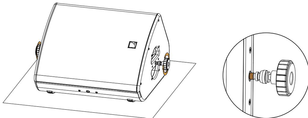
6. Lift the enclosure by the knobs and place it inside the U-bracket.
