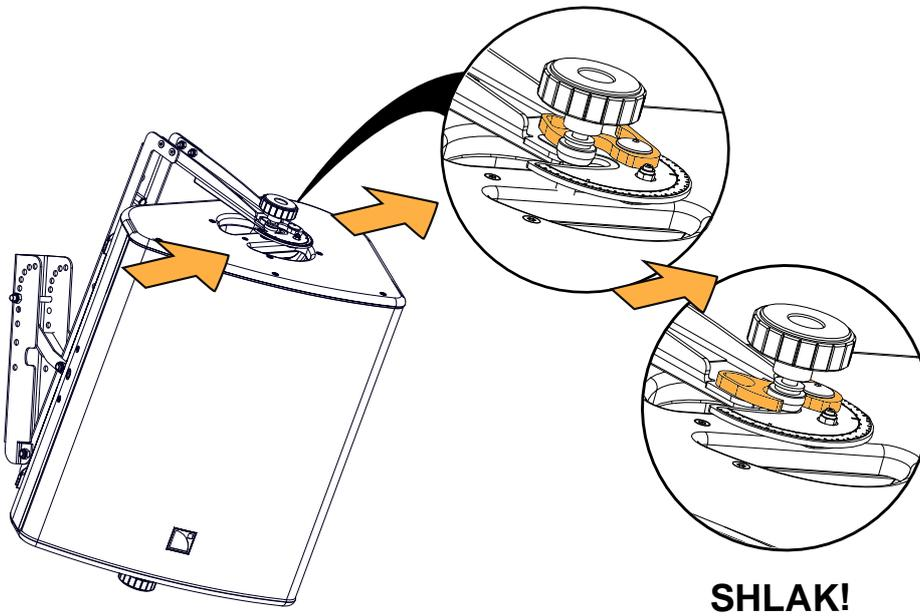
**8.** Set the azimuth angle.
