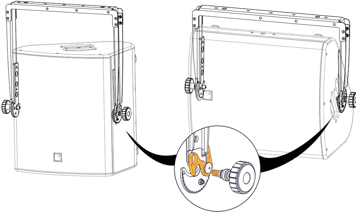
The threaded knobs feature a washer as a safety to avoid the accidental loosening of the knob.
