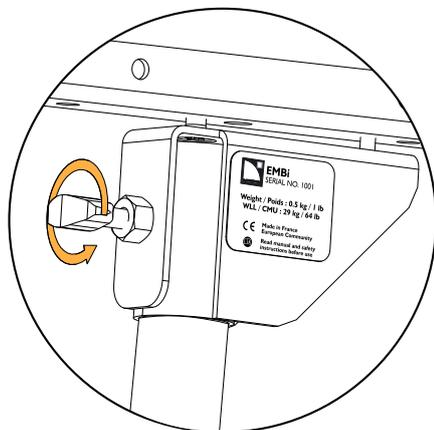
2. Remove the bracket from the enclosure.
