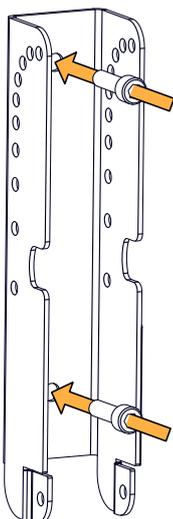
**2. Secure the U-bracket to X-UTILT.**
