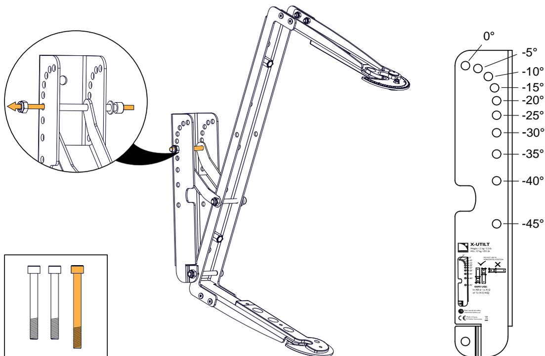
**5.** Drive the knobs in the inserts on the enclosure.
