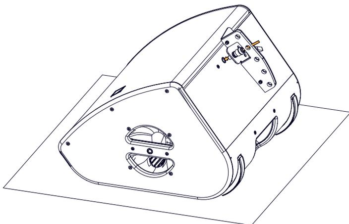
**3.** Rotate the X-BAR until perpendicular to the front grill.
