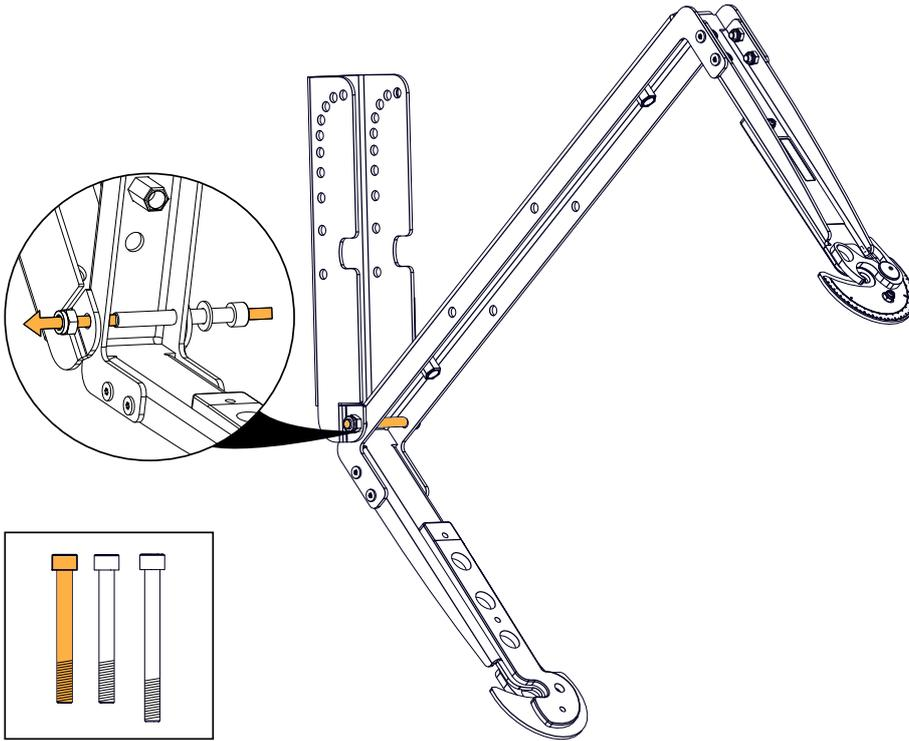
**3. Secure the rigging arm to the U-bracket.**
