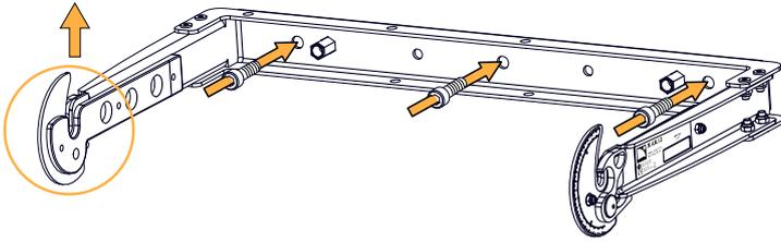
3. Lift the enclosure by the knobs and place it inside the U-bracket.
