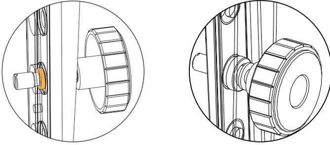
**3.** Tighten the knobs, reverse the assembly and mount it on a pole.
