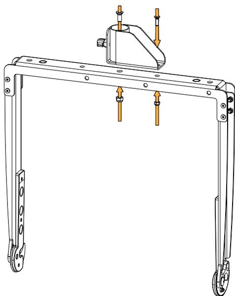
2. Secure the U-bracket to the enclosure using the additional holes.
