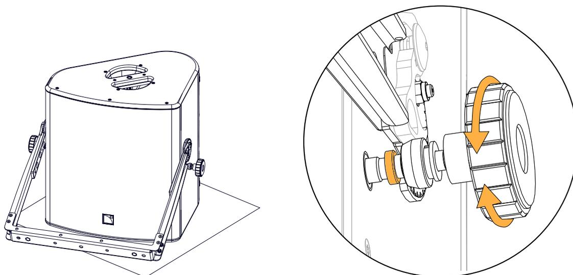
3. Push down until the knobs are locked inside the spring-lock mechanism.
