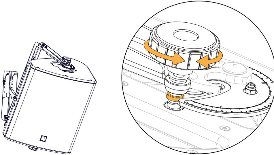
7. Push until the knobs are locked inside the spring-lock safety mechanism.
